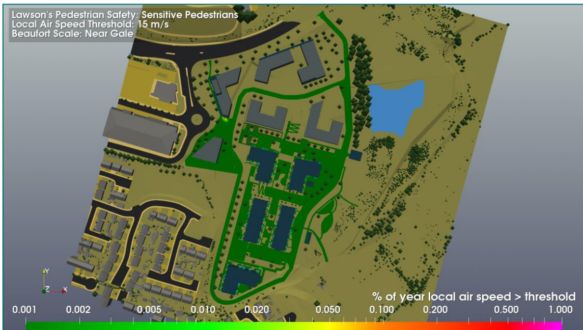
Figure 45: Sensitive Pedestrian Safety Criterion: Balconies: View from the south
