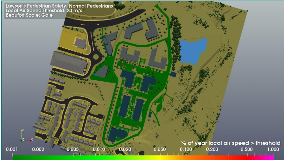
Figure 44: Normal Pedestrian Safety Criterion: Balconies: View from the south
