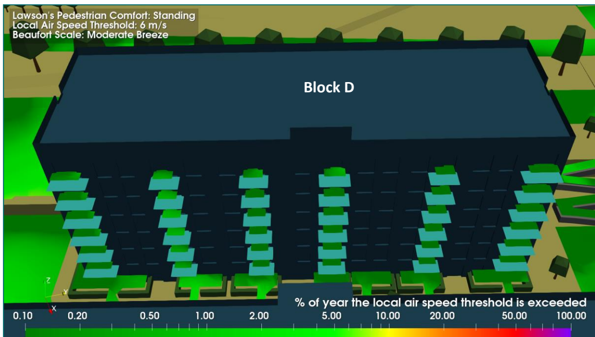
Figure 15: Standing Comfort Criterion: Balconies: Block D: View from the east
