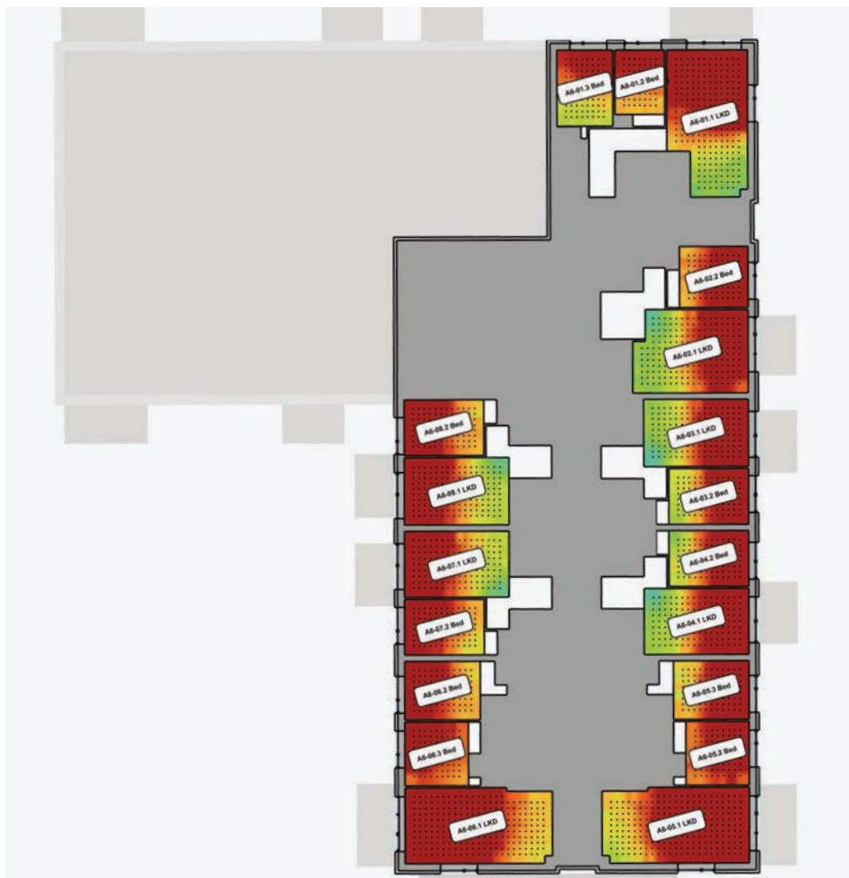
Figure 43: Block A - Daylight Provision and Annual Average Illuminance to all Habitable Rooms
