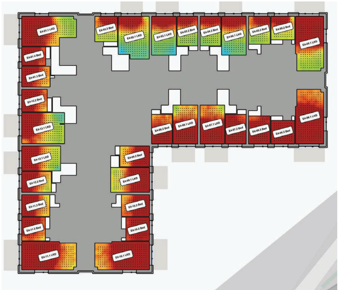
Figure 57: Block E - Daylight Provision and Annual Average Illuminance to all Habitable Rooms
