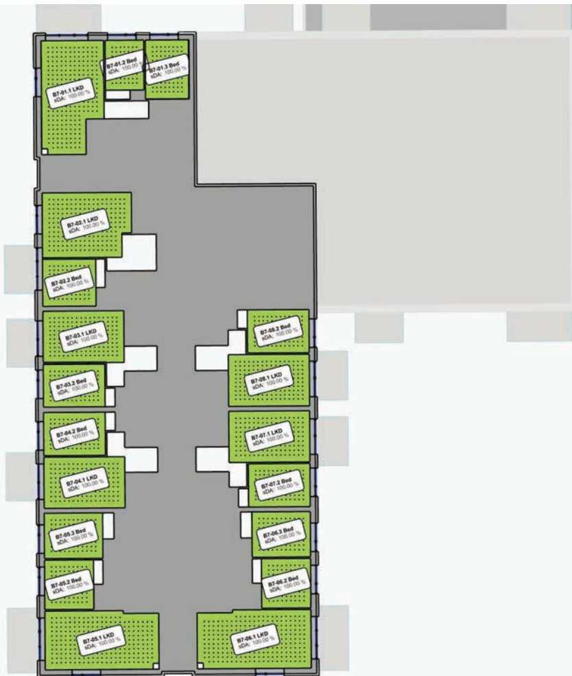
Figure 29: Block B - Floor plans indicating Daylight Provision to BS EN17037:2021+A1 Table NA.1
