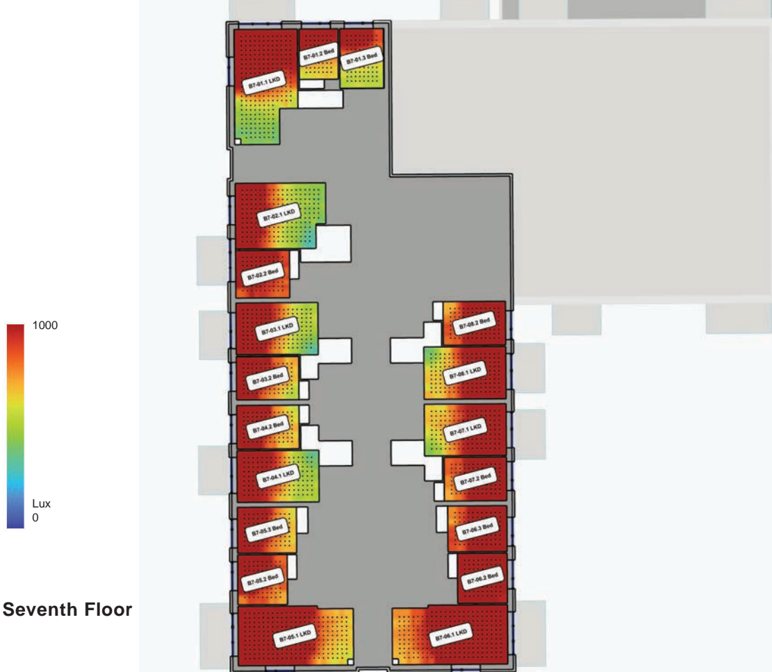
Figure 47: Block B - Daylight Provision and Annual Average Illuminance to all Habitable Rooms
