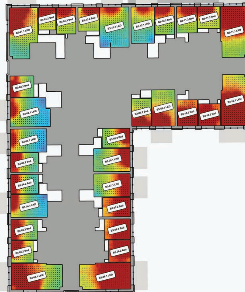
Figure 45: Block B - Daylight Provision and Annual Average Illuminance to all Habitable Rooms
